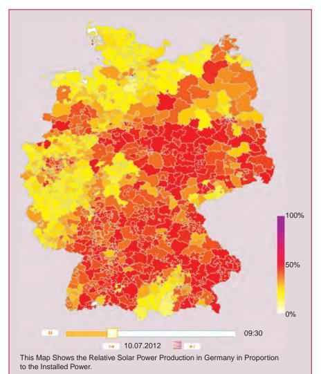
**figure 4.** The real-time estimation of the solar power production on a zip code level in Germany based on online data from inverters. (Source: energy & meteo systems.)
